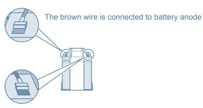
The blue wire is connected to battery cathode
